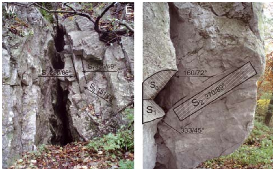
Obr. 9. Vyznačené diskontinuity pri vchode do jaskyne Malá skala Fig. 9. Marked discontinuity at the entrance to the cave Malá skala
